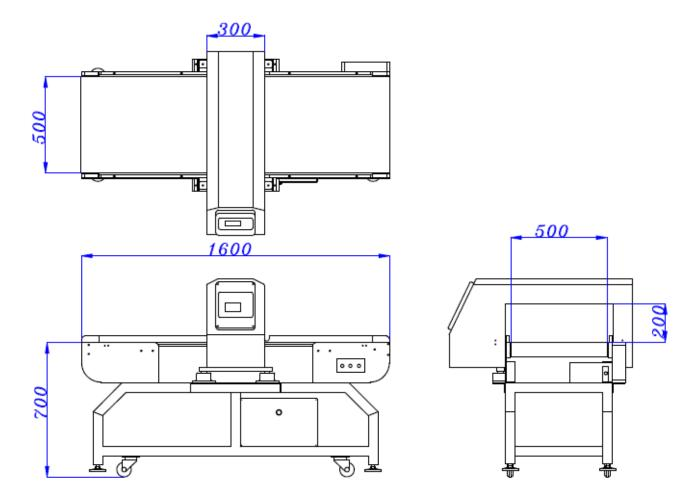
Metal Detector Machine with Flap Reject Dimension shown as below:
